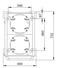
PD280N-TR-SC for plates Ø200...280mm
